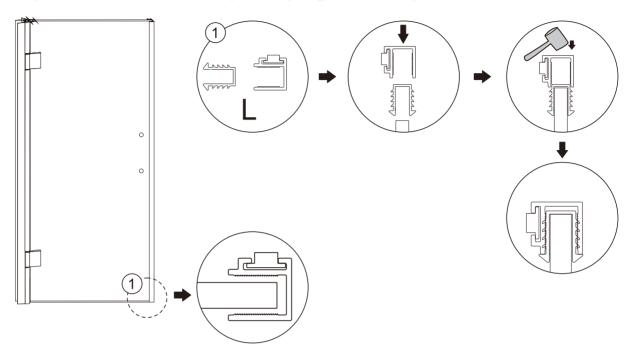
$\boldsymbol{R}\!\!:$  If need right opening, install according to procedures as below.
